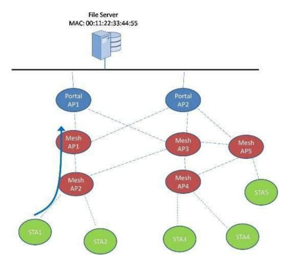
STA1 sent a data frame to Mesh AP2 destined for a local file server on the same subnet with MAC address 00:11:22:33:44:55. Mesh AP2's mesh forwarding algorithm determined that the frame should be forwarded through Mesh AP1.
