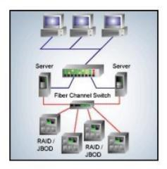
The SAN is a separate network that provides a storage repository that is attached to multiple host servers. SANs enable external storage to be shared by the servers without impacting system performance or the primary network.
