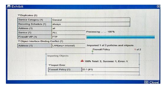
A. FortiManager already has Address LAN which has interface mapping set to "internal" in its database, it is contradicting with the STUDENT-2 FortiGate device which has address LAN mapped to "any".
