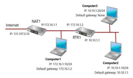
Computer1, Computer2, and Computer3 run Windows 10. Windows Defender Firewall is configured to allow ICMP traffic. RTR1 is a router.
