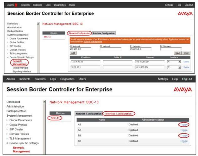
3. Click the Toggle link for both the A1 and the B1 interfaces. The Administrative Status for both A1 and B1 changes to Enabled:
