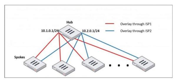
An administrator is deploying several spokes, including the BGP configuration for the spokes to connect to the hub.
