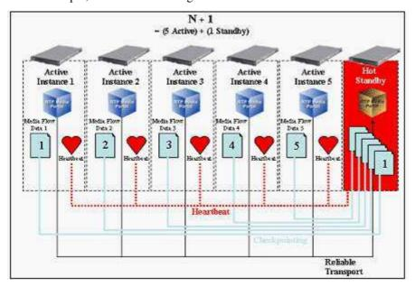
A.From a Gateway Controller (GWC), there is one cluster containing five active Border Control Point (BCP) 7200s and one standby BCP 7200.
