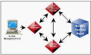
A.An alarm browser request is sent to the Database Manager (DBM), the DBM sends a request to the BCP to deliver alarm information back to the SMGUI.
