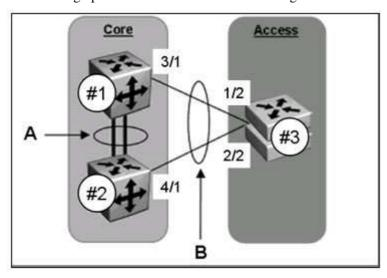
A.The ERS #1 Rx Process is enabled on all SMLT VLANs to monitor for ERS #3 SLPP packets.
