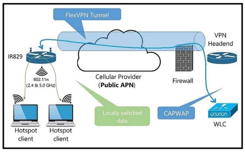
Refer to the exhibit. Which protocol is used to make a FlexVPN connection from a Cisco IR829 router to a headend router?
