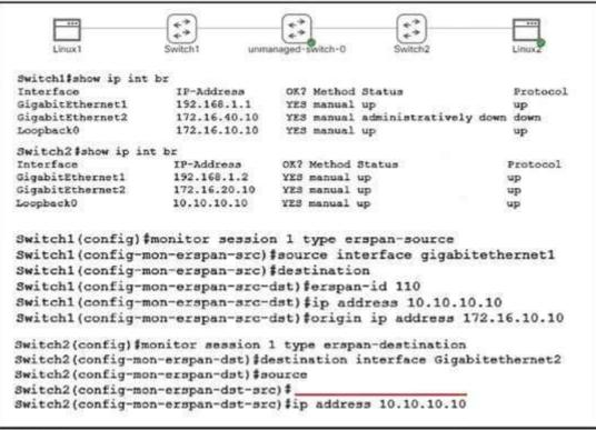
A. (config-mon-erspan-dst-src)# origin ip address 172.16.10.10
