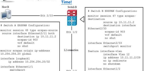
A. The session number of the source of ERSPAN spanned traffic must have a session ID of 47 for the traffic analyzer to receive the traffic.
