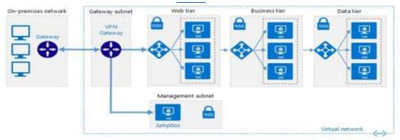
Scenario: Connect the New York office to VNet1 over the Internet by using an encrypted connection.
