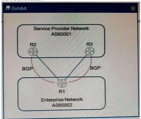
Referring to the exhibit, which mechanism is used to advertise routes from the enterprise network to the service provider network?
