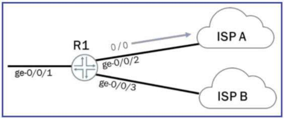
Your company has connections to two ISPs. Each ISP is in a separate routing instance. You need to advertise the 0.0.0.0/0 prefix from both ISPs to all your devices.
