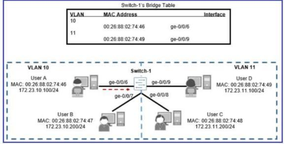
Switch-1 in the exhibit receives a packet from User A with a destination MAC address of 00:26:88:02:74:47. Which statement in this scenario is correct?
