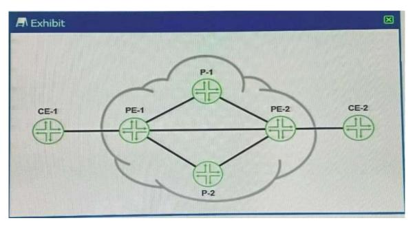
A Layer 3 VPN exists in the provider network and the CE devices are connecting to the PE devices using BGP. The PE devices are receiving BGP routes from the CE devices and the PE devices have the CE BGP routes in their respective routing tables. However, the remote CE devices are not receiving the BGP routes. Referring to the exhibit, what is the problem?
