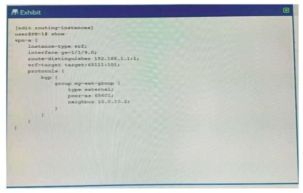
You have an established Layer 3 VPN between two PE devices. You are asked to only send certain routes from PE-1 over the VPN to the remote site while maintaining all the routes on the PE-1 device. You created a policy that matches the specific routes and then tags these routes with the appropriate target community values. In this scenario, which configuration changes must be made to satisfy the requirement?
