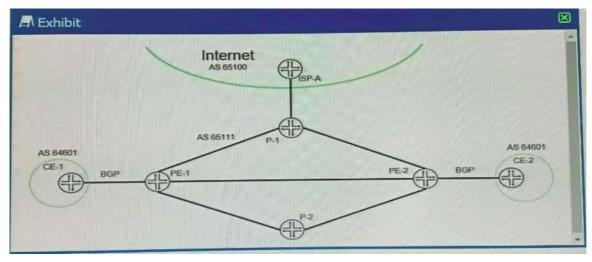
Referring to the exhibit, you have recently established a Layer 3 VPN between PE-1 and PE-2, connecting the two CE sites. Rowing information is being shared between sites and the customer has two-way communication After adding this VPN to your core network, PE-1 and PE-2 are no longer able to forward traffic to the Internet. In this scenario, what is the problem?
