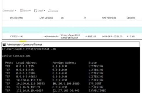
The exhibits show the collector state and active connections. The collector is unable to connect to aggregator IP address 10.160.6.100 using default port.
