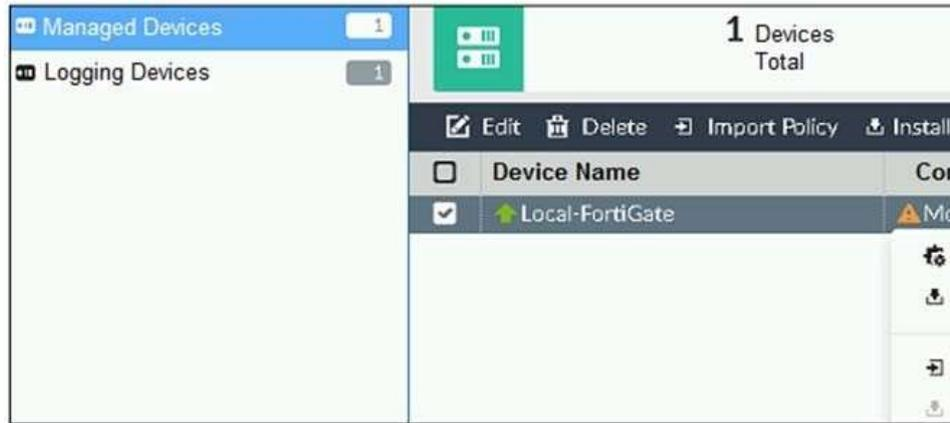
You are using the **Quick Install** option to install configuration changes on the managed FortiGate.
