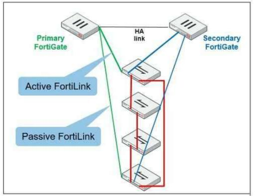
The exhibit shows two FortiGate devices in active-passive HA mode, including four FortiSwitch devices connected to a ring.
