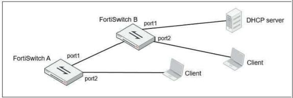
Given the network topology shown in the exhibit, which two ports should be configured as untrusted DHCP ports? (Choose two.)
